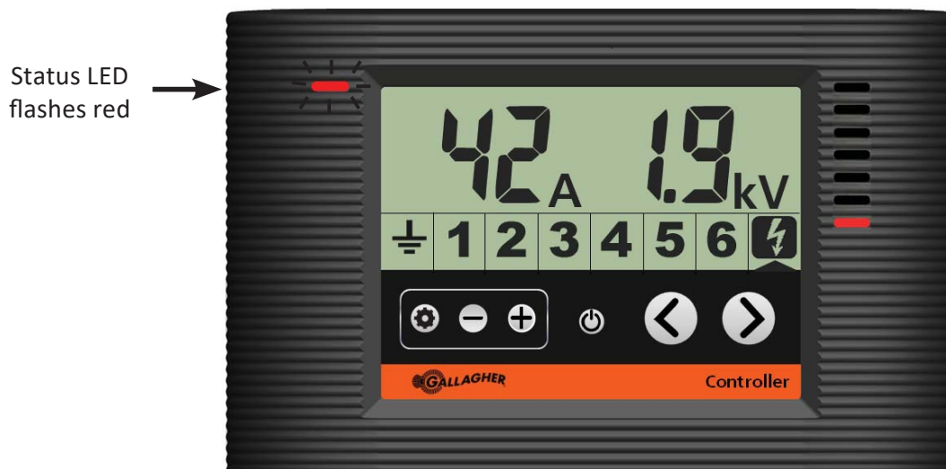
Controller showing the energizer in output alarm
