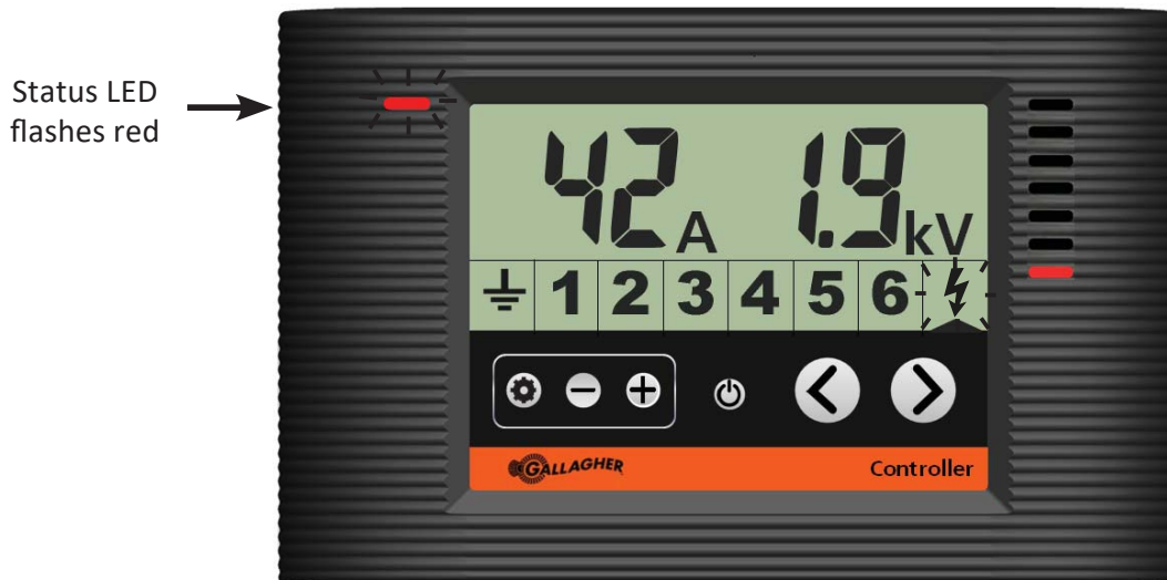
Controller showing the energizer in current alarm
